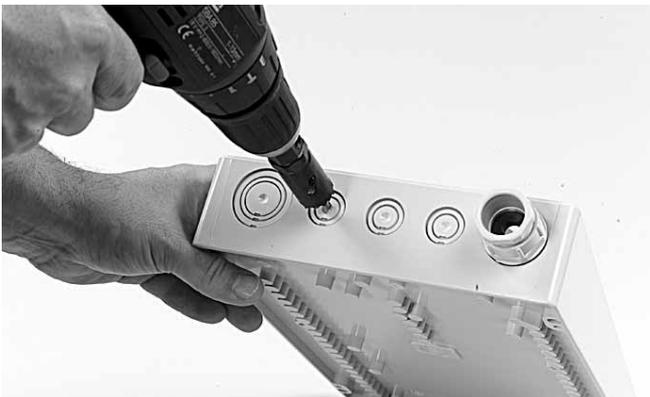
3.2.1 Drill or knock out the ports to be used, (cable in, port 1 - pigtails out, ports 2, 3, 4, 5).
