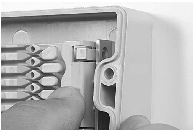
3.3.2. Pull on the long snapfit towards the profile till it clicks in the UMS bracket, start on the FAS block without leaving gaps between the plates.
