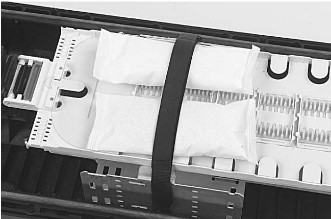
3.8.1 Place silica gel on the tray. When tower is fully loaded with trays, place silica gel at the side of the trays (between the trays and the Velcro).
