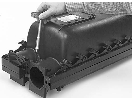
3.1.6 Loosen the bolts and lift the top part, revealing the closure bottom part. Leave the bolts in the top part of the closure.
