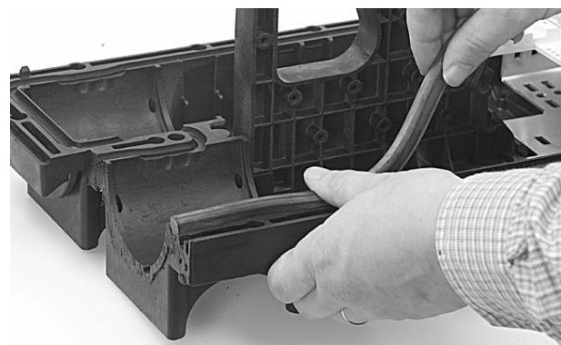
3.1.8 Insert the rubber seal in the groove starting at the open port.
