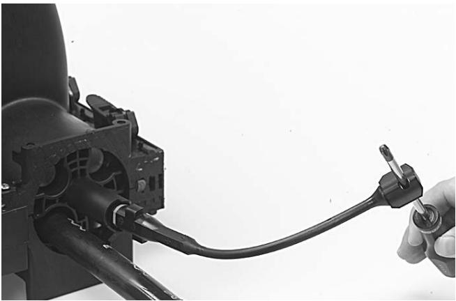
3.8.7 Turn the trigger of each gel block clockwise till the physical stop. Insert a screwdriver through the loop in the trigger to apply extra torque, if required.
